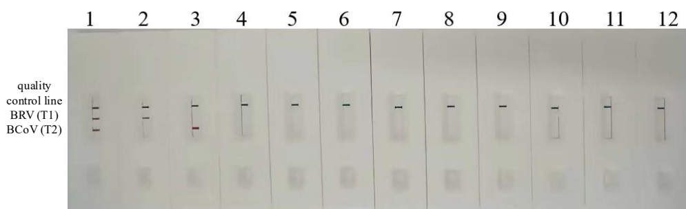
Figure 5. Dual LFD-RPA specificity test. 1: BCoV + BRV, 2: BCoV, 3: BRV, 4: BVDV, 5: IBRV, 6: BRSV, 7: E. coli , 8: C. perfringens , 9: S. typhimurium , 10: E. necatrix , 11: C. bovis , 12: negative control.
